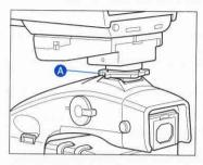
1. Install the SCA3952 adapter on the Metz flash, and put it on the camera then lock the flash in place using the locking knob on the flash shoe
