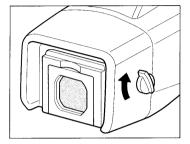
Turn the eyepiece shutter lever in the direction of the arrow.
