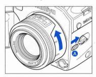
While sliding the lens release button back  ${\bf Q}$ , rotate the lens counter clockwise until it stops and lift it off.
