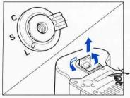
1. Lift the battery case lock lever, turn it counter clockwise and pull out the battery holder.
