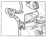
Put the neck strap through the camera's strap lugs as shown on the diagram and tighten it. For safety, check that the strap is securely fastened to the strap mount.
