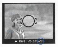
Press the AEL button in (a), the viewfinder LCD read-out displays the difference between the metered exposure value and exposure of a new composition. This is useful to check if an object with very different light level can be taken or not.
