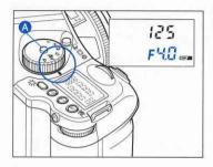
1. While pressing the exposure mode-setting dial lock release button in (a), turn the exposure mode-setting dial to the "Av" (aperture priority AE) position.
