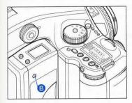
Make sure to pull the dark slide out, and half press the shutter release button while pressing the midroll film advance button in **3**.
