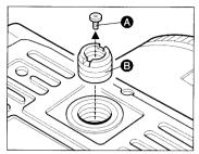
When using a tripod with 3/8 inch screw thread (instead of 1/4 inch screw thread) remove the small screw **(a)** from the tripod screw hole on the bottom of the body using a plus screwdriver, then use a coin to remove the tripod screw adapter bushing **(3)**.
