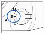
There are three focus modes: "S" (single focus mode), "C" (continuous focus mode) and "M" (manual focus mode).
