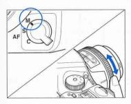
1. Turn the focus mode selector lever to "M" (manual focus mode) position. Turn the lens-focusing ring to focus. Half-press the shutter release button to meter exposure.
