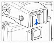
**1.** Remove the lens supplied with the finder by pulling it downward.
