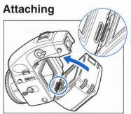
2. Match the groove on the magazine body coupler with the holder bracket (lower) of the camera body and snap the magazine into the body.
