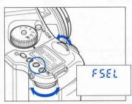
2. Press the key in for approximately two seconds, the main panel shows "Func". Turn the front or rear dial to select "FSEL".
