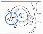
There are two shutter release modes: "S" (single-frame advance mode) and "C" (continuous advance mode). (See page 46.) When set to "L", the power is turned off.
