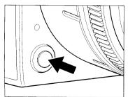
After focusing, press in the preview button. When using auto focus, the aperture is set to the displayed aperture while the button is pressed and the focus is locked.
