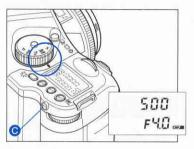
While the difference ③ between the set value and the metered value is displayed on the viewfinder LCD read-outs, press the AEL button ④ for approximately one second, the camera then changes the shutter speed to an appropriate level.
