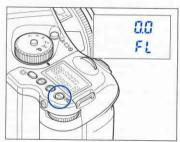
2. When the flash charge confirmation lamp lights, press the button in to show the "  $^{0.0}_{FL}$ " on the main LCD panel.
