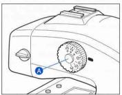
Turn the exposure compensation dial while pressing the exposure compensation dial lock release button in  $\triangle$  located on the right side of the viewfinder. The exposure can be adjusted within a range of  $\pm 3$  EV in 1/3 steps.
