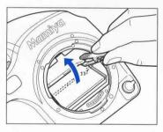
**4.** When installing the screen, pinch the protruding part of the screen using the screen holder, and put the screen on the screen frame.
