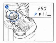
While pressing the exposure mode-setting dial lock release button in (a), turn the exposure mode-setting dial to "P" (program AE) position.
