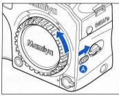
1. Remove the front body cap, just like you would remove a lens, by pushing the lens release button a backward and then turn the front body cap or the lens itself counter clockwise and lift out.
