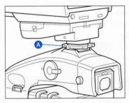
1. Install the SCA3952 adapter on the Metz flash, and put it on the camera then lock the flash in place using the locking knob on the flash shoe . Turn the shutter release mode selector lever to the "S" or "C" position, and turn ON the flash power switch.
