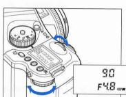
2. Turn the rear dial to set the desired aperture. The aperture value is adjusted in 1/2 stop increments.
