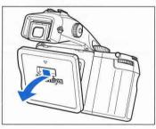
Remove the camera rear body cap while putting a finger into the notch and slide the cap down.
