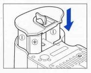
3. Return the battery holder to its case and lock it by turning the lever clockwise. Make sure it is firmly attached.
