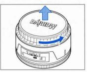
To remove rear lens cap turn it counter clockwise.
